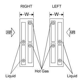
A typical two-section coil is shown.
