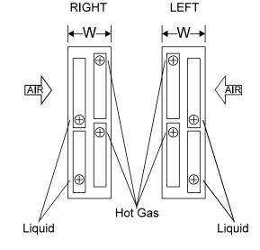
A typical two-section coil is shown.
