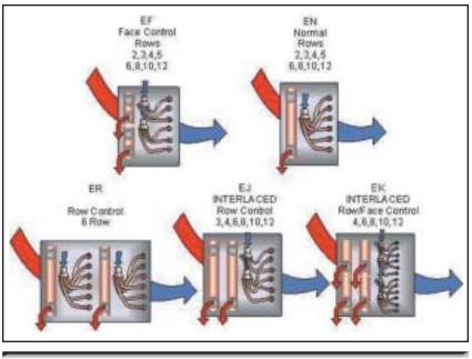
THERE ARE ALSO DIFFERENT TYPES OF EVAPORATORS THAT HAVE VARYING TUBE PATTERNS AND FIN SURFACES. THE TYPE OF EVAPORATOR CHOSEN CAN DETERMINE HOW MUCH MOISTURE IT CAN PULL FROM THE AIR. SOME OF THE DIFFERENT TYPES OF FINS AVAILABLE ARE A FLAT FIN, A CORRUGATED FIN, AND A SINE-WAVE FIN.
